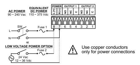
**Figure 2.4 Main Power Connections**
